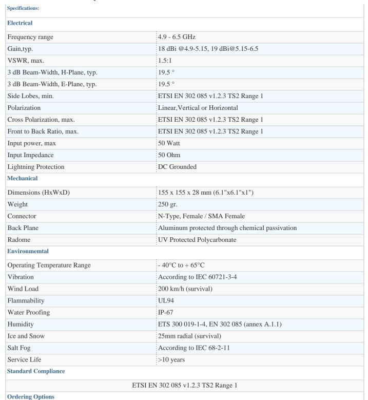
Antenna with N-Type, Female Connector Suited for MNT-23 (optional wall/pole adjustable mount) | MA-WA57-3HG1
