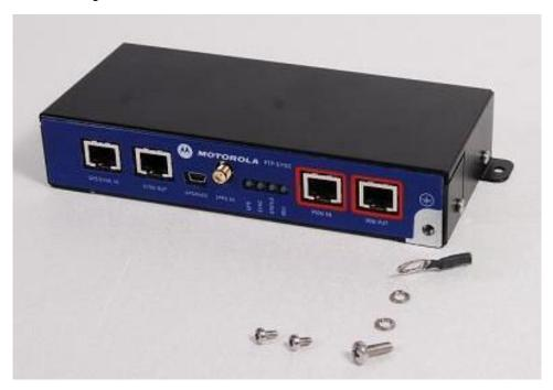
The kit contains:  $1 \times PTP$ -SYNC unit;  $1 \times M4$  pan screw;  $2 \times M4$  washers;  $2 \times M3$  (6mm) torx drive screws;  $1 \times M4$  unit ground (cable not supplied);  $1 \times Cat5e$  cable (length 1 meter).
