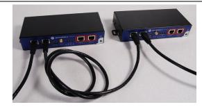
4 Connect the cable from the PIDU to the PIDU IN port. A suitable 1 meter cable is included in the PTP-SYNC kit.
