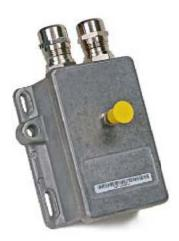
The PTP-LPU is a high-speed, high-current, solid-state device that is encased in a rugged metal case designed to hold up against ice, snow and rain and to withstand winds up to 150 mph (242 kph). The projected operational life of a PTP-LPU is 10 years, even when continually exposed to the elements. Because of its small form factor and minimum number of components, the unit is easy to transport and install. Plus, the cost-effective PTP-LPU is affordably priced.
